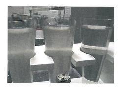
Imhoff Cones (pictured to the left) show the results of the treatment process at the wastewater treatment facility. The first cone is a sample of the water as it enters the plant. The second cone shows the results of passing through the primary treatment process. The third cone shows the final 'effluent' sent to the Androscoggin River after it passes through the secondary treatment process.
